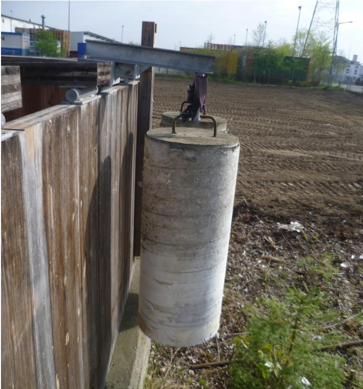
Figure 4 weight made from concrete for test specimens with constant moment-loading (series 1)
