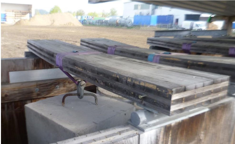
Figure 6 test specimens with single point loading (series 3)
