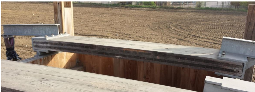
Figure 3 test specimen with constant moment-loading (series 1)
