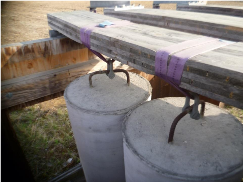
Figure 5 test specimen with third point loading (series 2)
