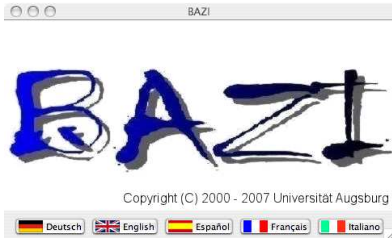
Fig. 1: Bazi’s welcome screen. When invoked through the command java -jar bazi.jar , Bazi prompts the user for language selection. With an appropriate switch appended to the calling command, the prompt is shortcut.
